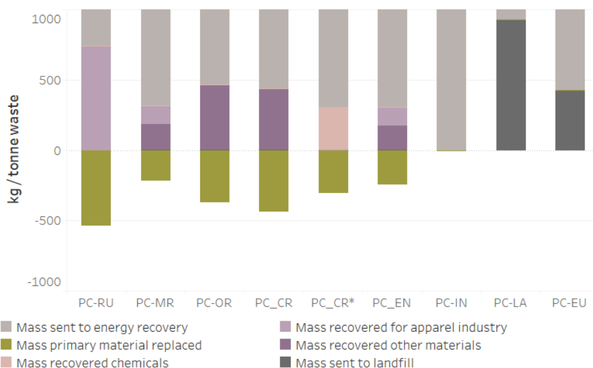
Figure 26. An overview of mass balances in the investigated scenarios for the management of 1 tonne of polycotton waste (PC) via re-use (RU), mechanical recycling (MR), open-loop recycling (OR: production of insulation material), dissolution in two variants: 1) dissolution of cotton and recovery of polyester (CR) and 2) dissolution of polyester and recovery of cotton (CR*), enzymatic recycling (EN), incineration (IN), landfilling (LA) and combination of the last two (EU) (it is referred to Table 7 for a description of the different treatment scenarios and technologies). The category mass recovered textiles for apparel includes re-used textiles and spinnable fibers from mechanical recycling that could potentially be used in the apparel retail industry and contribute to avoiding production of virgin textiles. The category mass recovered other materials includes short fibers and other products (e.g. insulation material) that can replace other materials such as e.g. virgin insulation. The category mass primary material replaced shows to what extent the products from the selected scenarios can replace their virgin counterpart.
